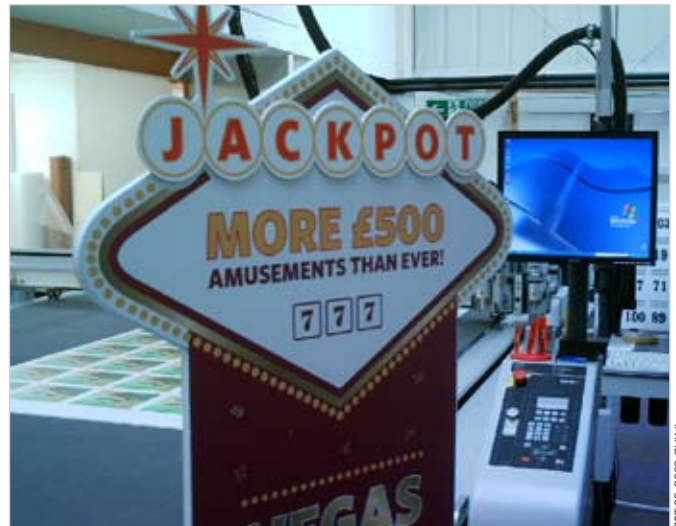
The „jackpot“ part made of 3mm expanded PVC for a 3D-effect.
