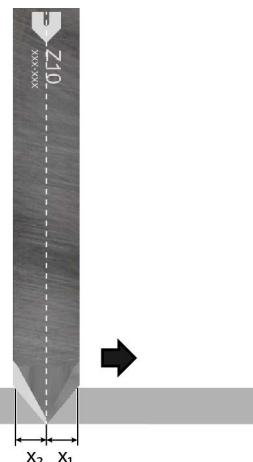
**Sample calculation Z20****Formula**  $x = 1.2 + 0.11 \times Tm$ **Cutting depth**  $Tm = 10.2 \text{ mm}$ **Pre-cut:**  $x_1 = 2.322 \text{ mm}$ **Sample calculation Z11****Formula**  $x_{1,2} = 0.58 \times Tm$ **Cutting depth**  $Tm = 5.2 \text{ mm}$ **Pre-cut:**  $x_1 = 3.016 \text{ mm}$ **Post-cut:**  $x_2 = 3.016 \text{ mm}$ **2.1.7 Blade Types**
