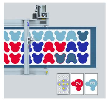
In this example, five suction cups are activated to remove the part. The end effector automatically positions itself correctly for easy removal of the cut part.
