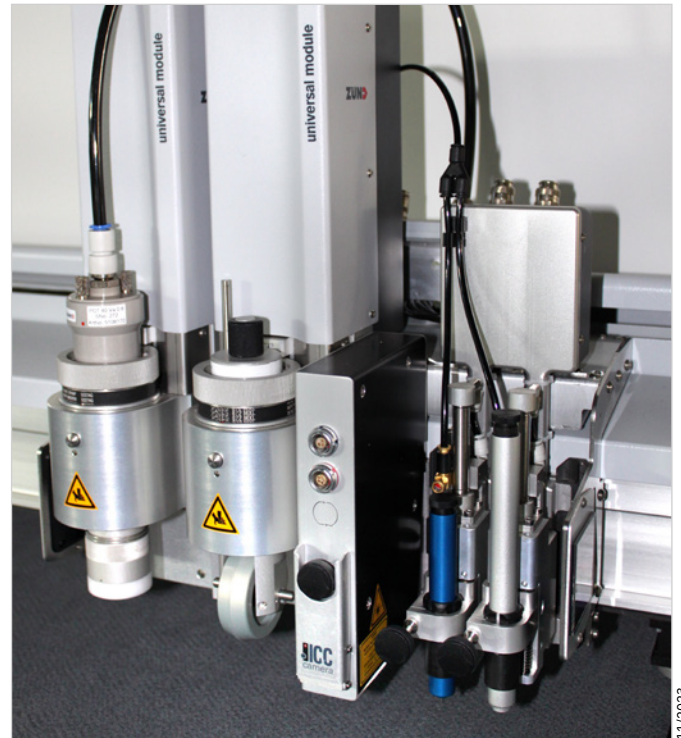
Fully equipped module carrier with 2 UM, ICC Camera and MAM-D.
