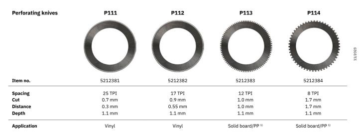
Depending on the material thickness, a very high contact pressure is required to perforate PP (Z-axis force > 10 kg). Tip: The UM-ZP Universal Module is ideal as a carrier for creasing and perforating tools.
