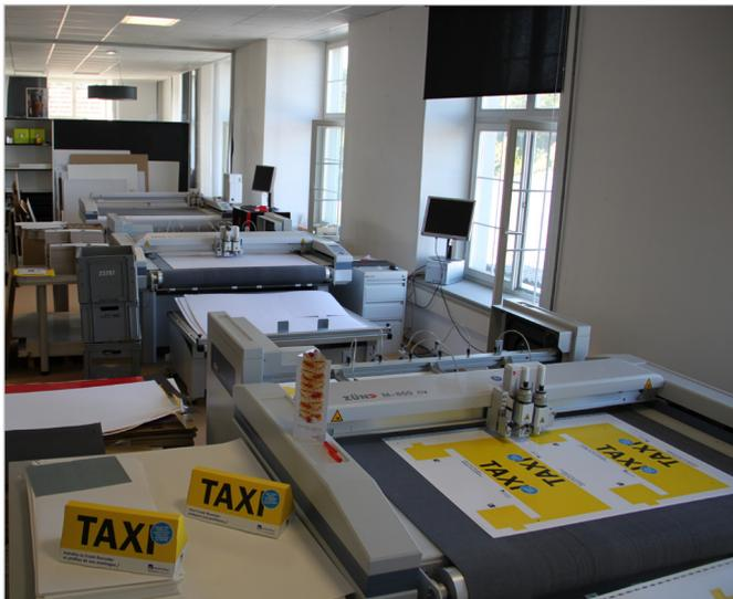
View of the production floor with 3 Zünd M-800 cutting systems lined up.
