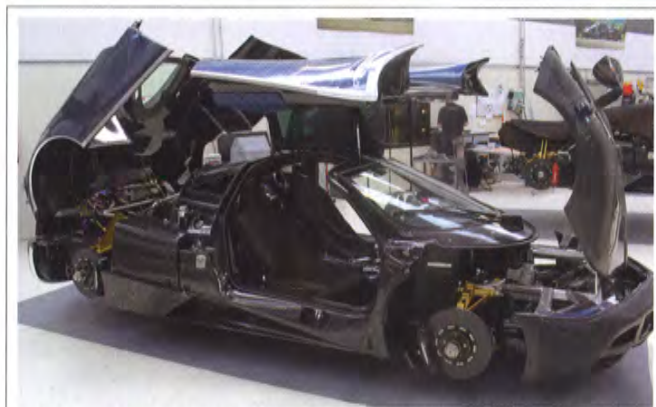
Each Pagani chassis is constructed from precisely 240 carbon-based composite components
